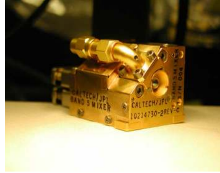
Fig. 2. A general view of the 1.2 THz mixer we delivered for integration in HIFI of Herschel Space Observatory. The silicon lens is visible at the mixer front. The SIS mixer chip is mounted at the back side of the lens. The mixer structure is solid and sustains well the vibrations levels possible at launch. The same design will be used at SOFIA. For more design details see [8].
