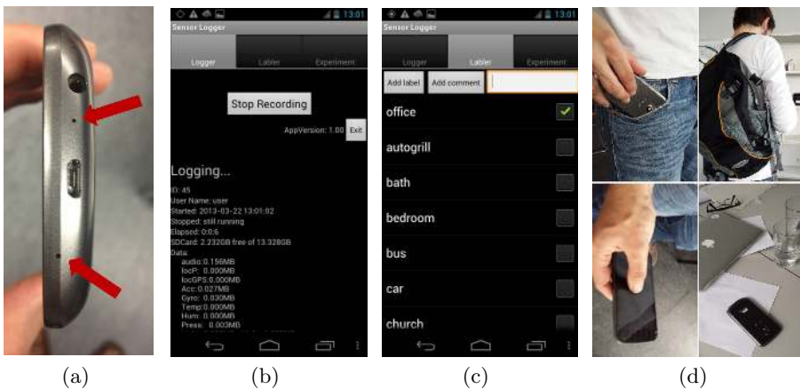
Fig. 2. (a) The modified Samsung Galaxy Nexus with added temperature and humidity sensors, (b, c) screenshots of the Android application for data gathering, and (d) an illustration of different phone wearing-contexts for a user during its daily-pattern (pocket, backpack, hand, table)
