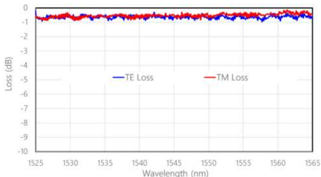
Fig. 19. Insertion loss performance of the polarization beam splitter/combiner across the C band of the SSMF.
