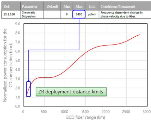
Fig. 12. Normalized power consumption for CD compensation as a function of fiber length.
