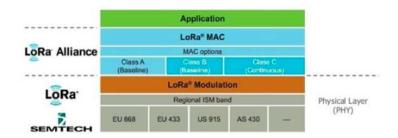
Figure 2.8: Relation between LoRa, LoRaWAN and OSI model[33]
