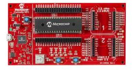
Figure G.3: Microhip Curiosity HPC development board (obtained from Microchip's website)
