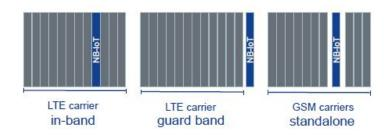
Figure 2.2: Configurable modes for NB-IoT deployment [13]
