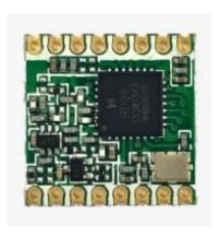
Figure F.3: HopeRF RFM96W LoRa modem [72]
