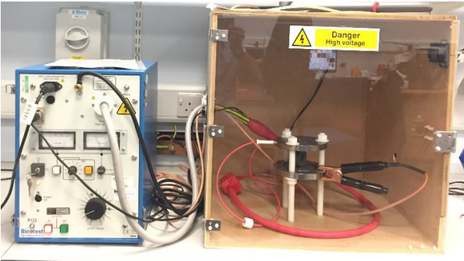
Figure 10. 30 kV power supply and floating point PD emulation cell.
