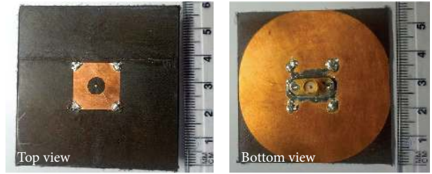
FIGURE 8: Manufactured prototype based on Rogers Duroid 5880 substrate.
