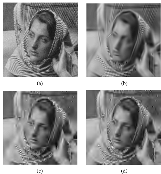
Fig. 10. Barbara ( 256 \times 256 ) encoded at 0.12 bpp. (a) Original. (b) MP, 21.35 dB. (c) JPEG2000, 21.23 dB. (d) SPIHT, 21.29 dB.
