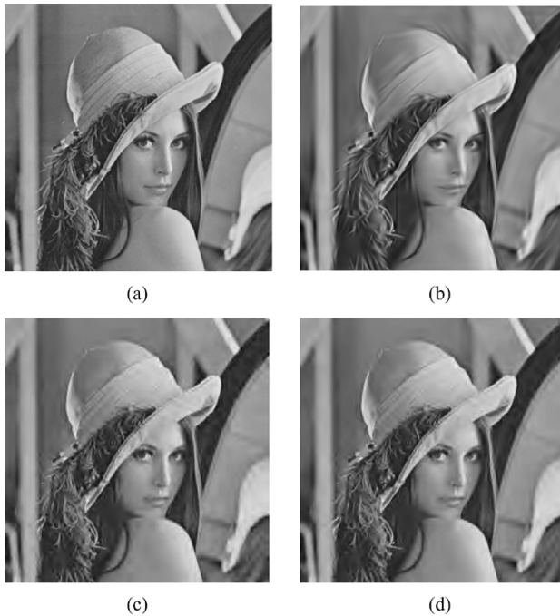
Fig. 6. Lena ( 256 \times 256 ) encoded at 0.35 bpp. (a) Original. (b) MP, 30.3626 dB. (c) JPEG2000, 30.7940 dB. (d) SPIHT, 31.3471 dB.
