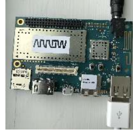
(b) Qualcomm Snapdragon 400 Mobile Development Board used for the multi-task deployment.
