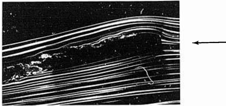
Figure 16. Flow About an NACA 23012 Airfoil at an Angle of Attack of 14 Degrees and a Reynolds Number of 123,800 (From Reference 102).
