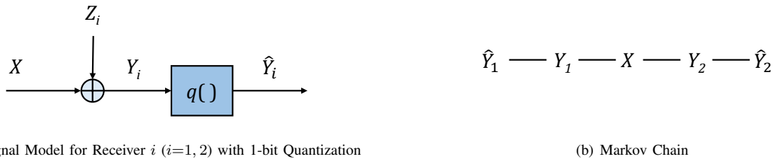
Fig. 2. (a) Signal model showing additive noise and quantization at receiver i and (b) Markov chain representation of transmitted and received signals.
