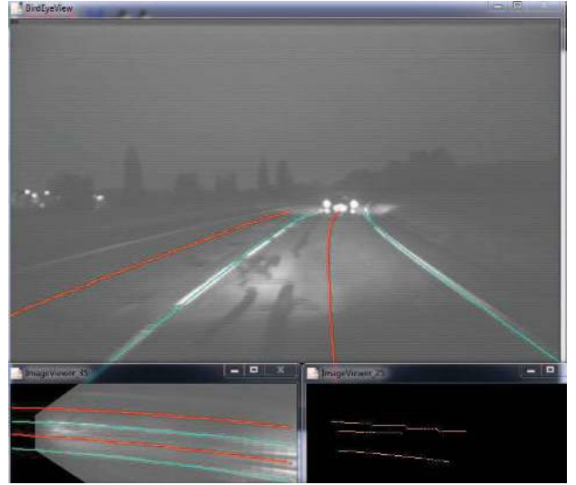
Fig. 6. Lane detection and tracking result - Cyan lines are the current lane boundaries. Red lines are the lane centers. Bottom figures are bird eye view images: the right one is a binary image containing extraction points.
