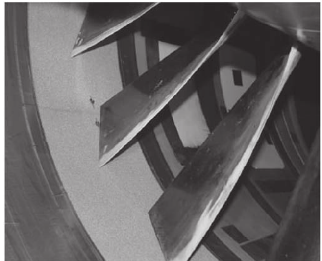
Fig. 11 FML spool installed over the rotor.
