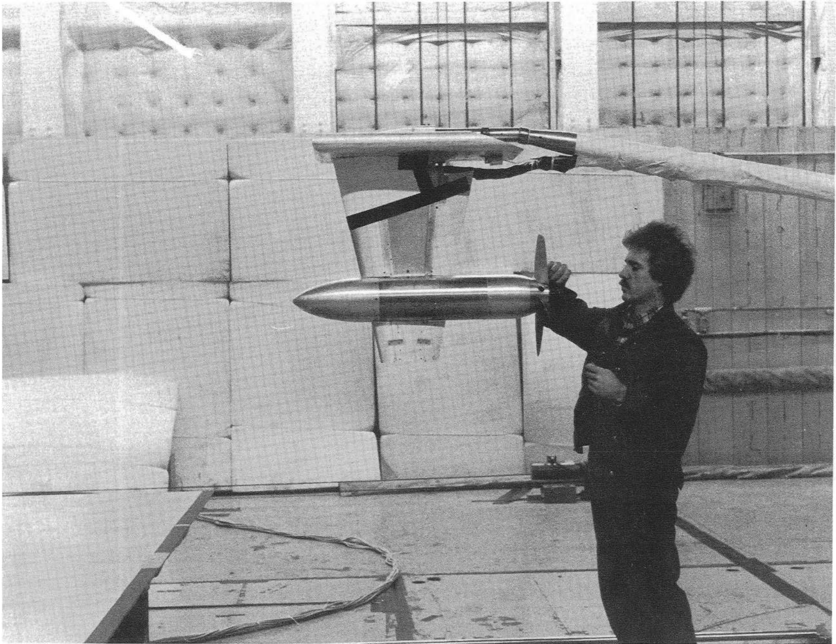
Figure 3.- Photograph of pylon-mounted pusher propeller/nacelle.
