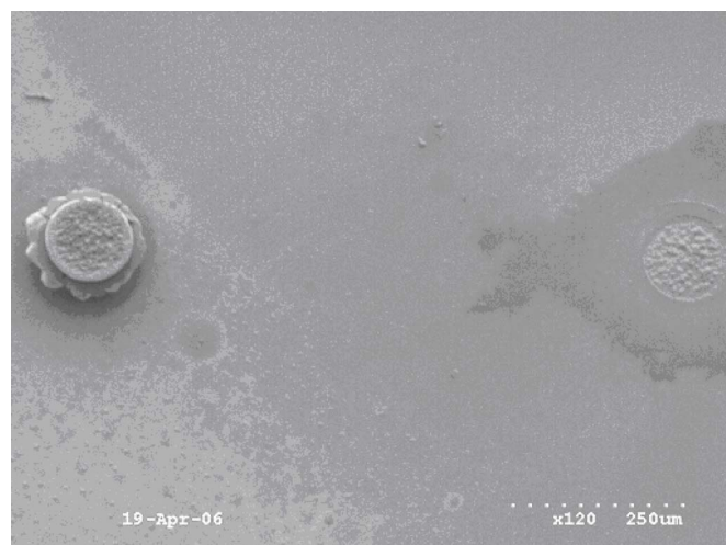
Figure 3. SEM picture of a sheared off substrate.
