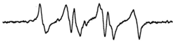
Figure 15 EPR spectra of alkoxy radical generated by soybean lipoxygenase and linolenic acid using DMPO as the spin trap (Dikalov & Mason 2001).
