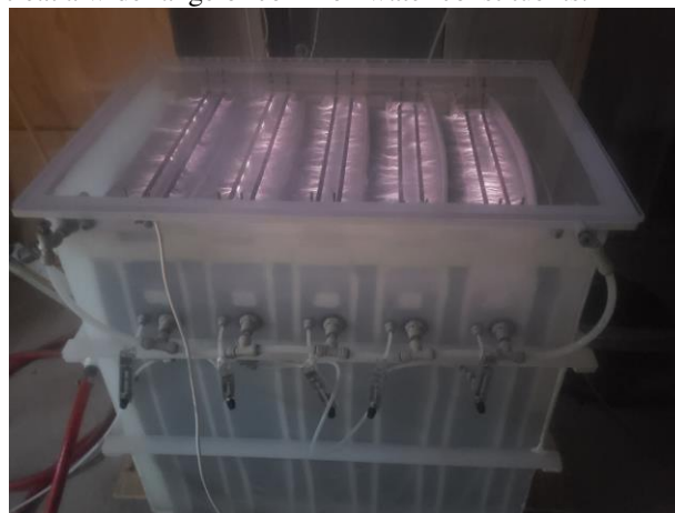
Fig IV.2. A commercial 10 gpm water treatment system based on electrical discharge plasma (courtesy of Plasma Research Laboratory, Clarkson University).
