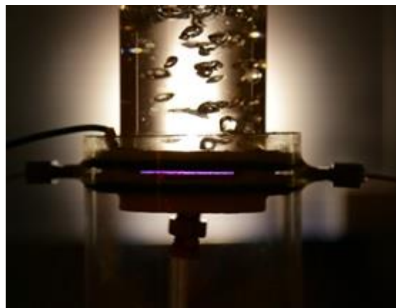
Fig. IV. 1 A dielectric barrier discharge for nitrogen fixation in water. The plasma is in direct contact with the water surface. To increase the residence time and the surface area to volume ratio, air is flown through the plasma and bubbled into a 500 ml water column. (courtesy of Plasma for Life Sciences Laboratory, North Carolina State University).
