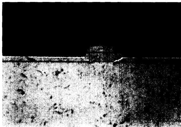
FIG. 2. Photomicrograph of the cross section of an embedded double-heterostructure laser grown through a window opened in a GaAlAs-GaAs mask.
