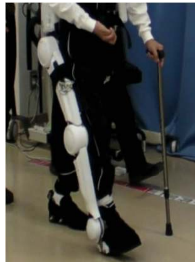
FIGURE 9: Single-leg version of HAL robot (picture courtesy of Professor Sankai, CYBERDYNE Inc./Univeristy of Tsukuba).
