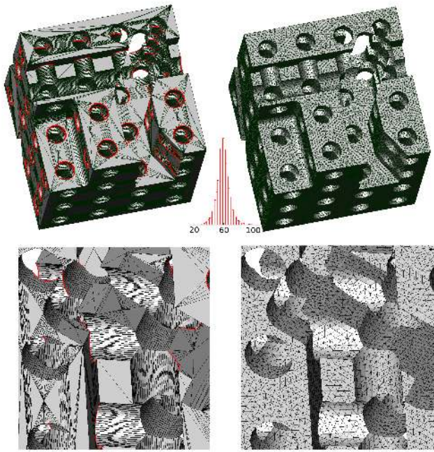
Figure 10: Left: 'nastycheese' dataset (borders shown in red); Right: isotropic remesh and angles histogram. Bottom: closeup. Sharp features are naturally reconstructed by L_2 -CVT with normal anisotropy, without needing to detect or tag them. Timing: 215 s.
