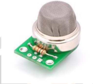
Figure 3: The configuration of MQ6 gas sensor
