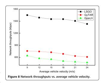
LSGO selects a set of candidate nodes to forward the packet, so that it has a high probability of successful transmission of the packet, and consequently, the network throughput is improved.
