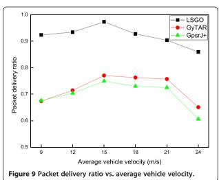
and then drops with the increase in vehicle velocity. It is because that, for one node, the possibility of appearing effective neighbors becomes higher due to vehicles moving. However, when the vehicle speed continues to increase, the connectivity between vehicles deteriorates with this change, and the bad link quality results in a lower delivery ratio.
