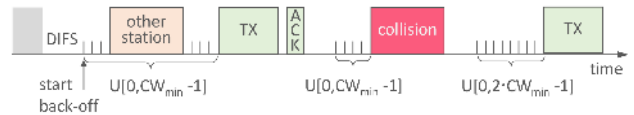
Figure 2: Wi-Fi operation – decentralised CSMA/CA based channel access; stations transmit when channel is sensed idle, after a back-off procedure.
