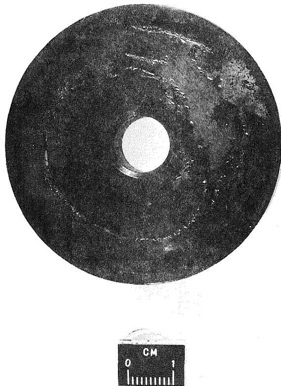
Figure 8. - Sputtered MoS 2 film on copper surface.
