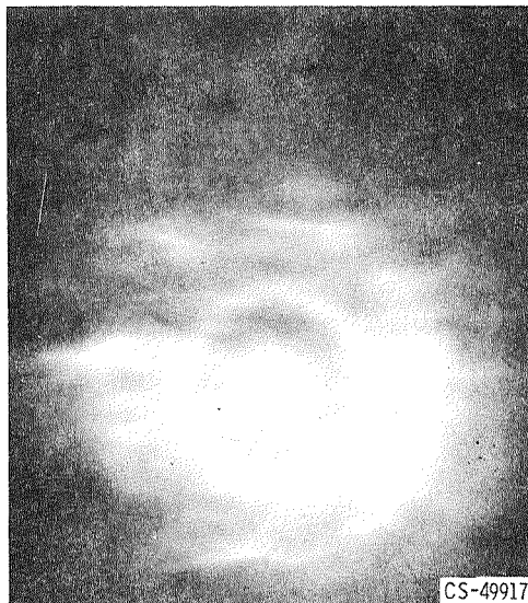
Figure 6(a). - Electron diffraction pattern of sputtered MoS 2 film.
