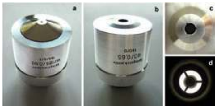
Fig. 7: Mirror objectives Zeiss Jena. a: W 120/0.90 160/0.17 (katadioptric water immersion). b-d: 40/0.65 160/0 (katoptric system)
