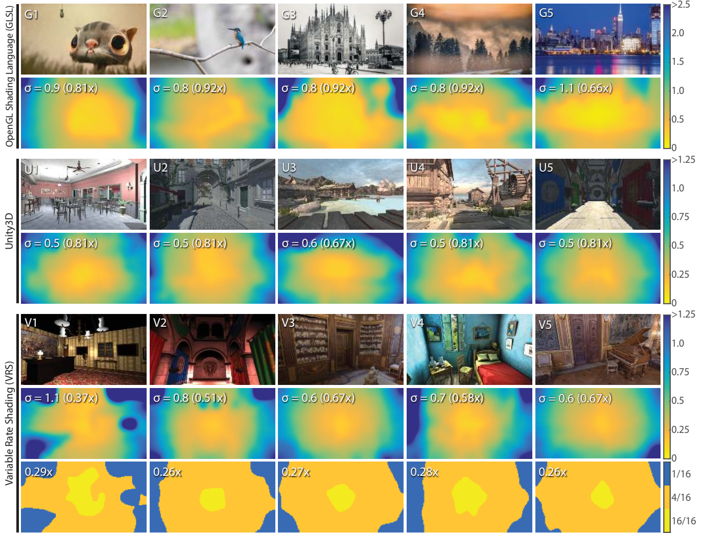
Fig. 10. Sample inputs and predictions from the implementation of our model on different platforms. The gaze position is assumed to be at the center of the screen for comparison. The color maps show the predicted standard deviations ( \hat{\sigma}_s ) in the second row for each platform. \hat{\sigma}_s = 0 represents a requirement for rendering in the native display resolution whereas larger values represent rendering in a lower resolution. Average value of each \hat{\sigma}_s map is shown in the top-left corner and the numbers in parentheses are the estimates of the resolution reduction with respect to the standard foveated rendering. They are computed as the ratio of average sigma values from a standard foveated rendering implementation and our method. The standard foveation parameters are selected from the ground truth of text patch in our training set (Image 9 in Figure 5), which represents a visual content with high spatial frequencies. The third row in Variable Rate Shading shows the optimization of rendering resolution using our model, which is color coded according to different sampling rates supported by VRS API. The number in the top left corner represents the fraction of pixels which are actually shaded for each one of these frames.
