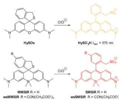
Fig. 92 Structure and spirocycle ring opening reactions of HySOx and MMSiR with hypochlorite.
