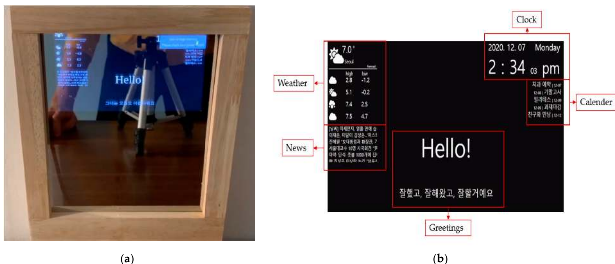
Figure 6. The smart mirror LUX: (a) the front view model of LUX, and (b) the display view of LUX, including weather, clock, calendar, and news.
