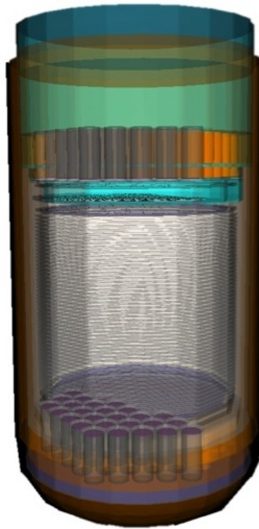
FIG. 3. The LUXSim rendering of the internal components of the LUX1.0 detector. The simulated detector includes the major components that affect the optical response and background, including the Hamamatsu R8778 PMTs, the reflective PTFE surfaces, and the grid wires and frames. All 122 PMTs are present in the simulation, although the visualization hides some of them. Compare to Fig. 1.
