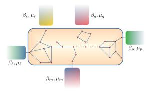
FIG. 1. A system on a lattice of arbitrary geometry and dimension coupled to at an arbitrary number of sites to thermal baths which can all be at different temperatures (inverse temperatures, say,  $\beta_{\ell}, \beta_{m}, \beta_{p}, \beta_{q}, \beta_{r}$ ) and chemical potentials (say  $\mu_{\ell}, \mu_{m}, \mu_{p}, \mu_{q}, \mu_{r}$ ).
