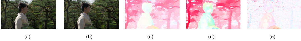
Figure 7. Visualized results of compressing the Kimono sequence using Add MAMVP-Net model with \lambda = 16 . (a) The reference frame \hat{x}_5 . (b) The original frame x_6 . (c) The original MV v_6 . (d) The predicted MV \bar{v}_6 . (e) The MVD d_6 .
