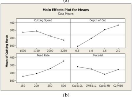
**Figure 9.** Diagrams showing the responses of (a) S/N ratios and (b) data means when evaluated against the cutting parameters which optimise the cutting force [50].
