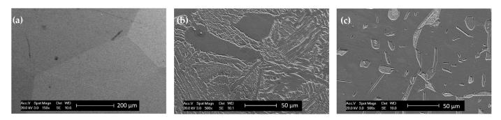
**Figure 3.** SEM micrographs on longitudinal sections showing the microstructures of (a) CuZn42, (b) CuZn38As and (c) CuZn36, after the selected heat treatment condition [25].
