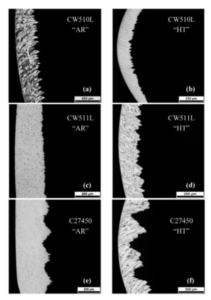
**Figure 7.** Optical micrographs showing the morphology of chips generated during the machining process of (a) CuZn42, (c) CuZn38As, (e) CuZn36 alloys before heat-treating (AR) and (b) CuZn42, (d) CuZn38As, (f) CuZn36 alloys after the heat-treatment process, HT [25].
