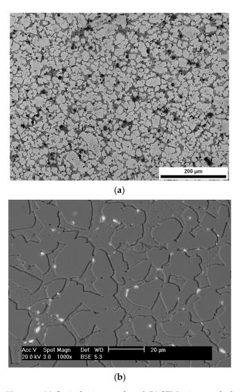
**Figure 1.** (a) Optical micrograph and (b) SEM micrograph showing the typical microstructure of CuZn39Pb3 (CW614N) brass [50].
