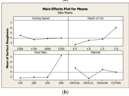
**Figure 10.** Diagrams showing the responses of (a) S/N ratios and (b) data means when evaluated against the cutting parameters which optimise the surface roughness [50].
