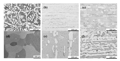
**Figure 2.** Optical micrographs of the (a) CuZn42, (b) CuZn38As, (c) CuZn36 alloys before heat-treating and (d) CuZn42, (e) CuZn38As, (f) CuZn36 alloys after the heat-treatment process [25].
