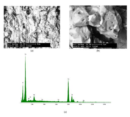
**Figure 5.** (a,b) Backscattered Electron (BSE) micrographs showing the fracture surface of a brass component showing intergranular morphology, (c) EDS spectrum of the fracture surface showing the presence of oxides. See Reference [93].
