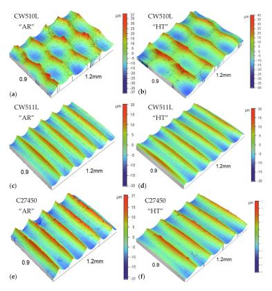
**Figure 8.** Surface topography derived from profilometric measurements: (a) CW510L, as received, (b) CW510L, heat-treated, (c) CW511L, as received, (d) CW511L, heat-treated, (e) C27450, as received and (f) C27450, heat-treated [25].
