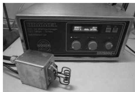
Figure 11. An inductive system used for the machine-assisted heating of a continuous-flow reactor column. Reprinted from Ref. [54a].
