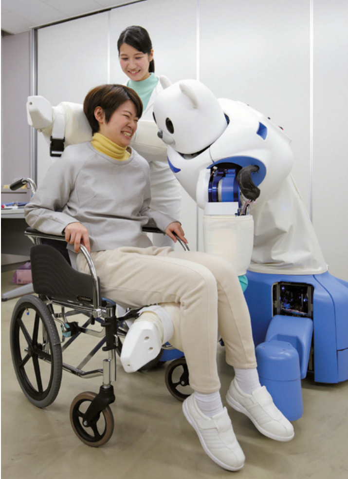
'Robear' is designed to help to care for ill or elderly people.
