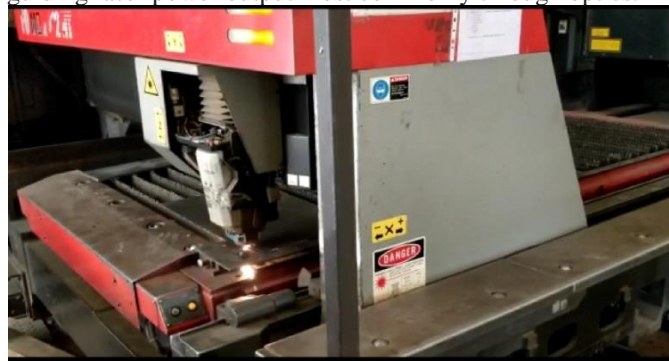
(a) Laser Cutting of the Job in progress
