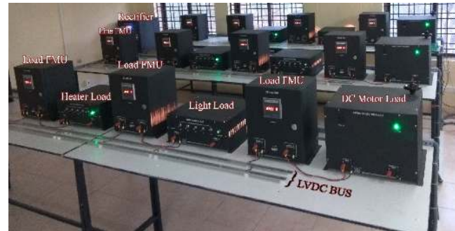
Figure 2. Real-time prototype distribution system
