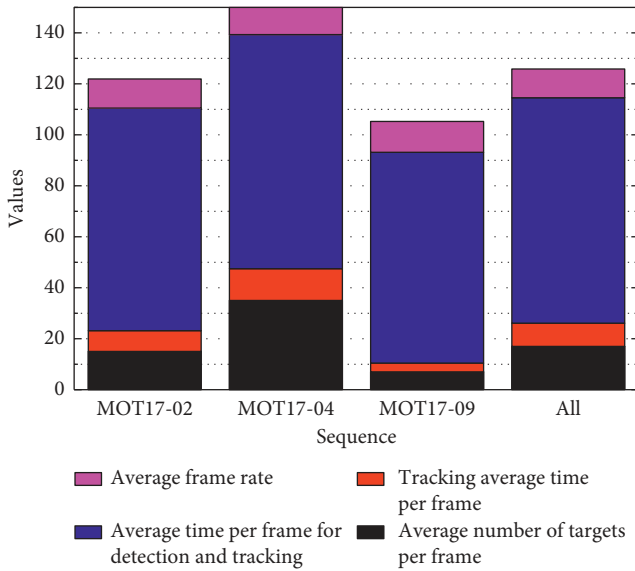
FIGURE 8: Test elapsed time and average frame rate of multitarget tracking algorithm on MOT17 dataset.
