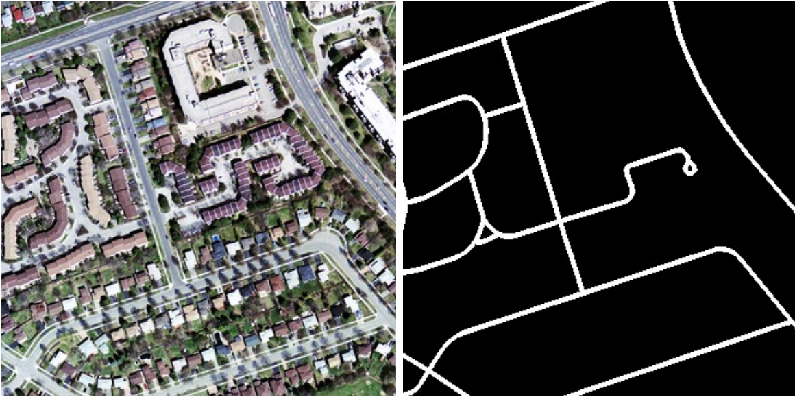
Figure 3.1: Sample aerial image (left) and a binary map (right) denoting the location of roads.
