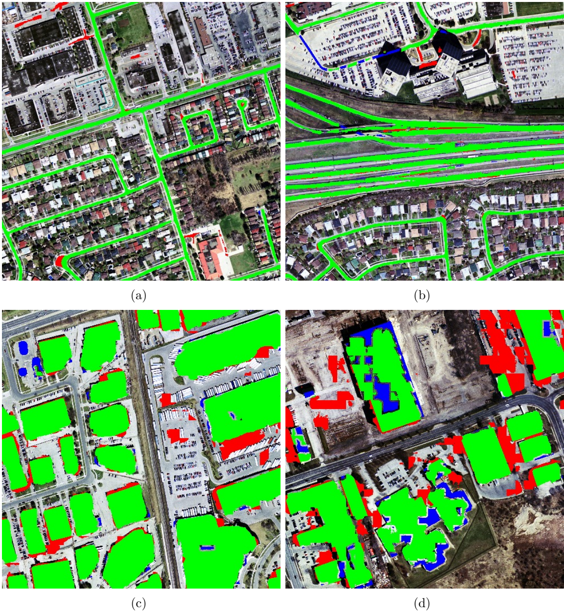
Figure 3.9: Visualizations of neural network predictions on road and building detection tasks. Green pixels are true positives, red pixels are false positives, blue pixels are false negatives, and background pixels are true negatives. Figures 3.9(a) and 3.9(b) show predictions on the Toronto Roads test set. Figures 3.9(c) and 3.9(d) are predictions on the GTA Buildings test set.
