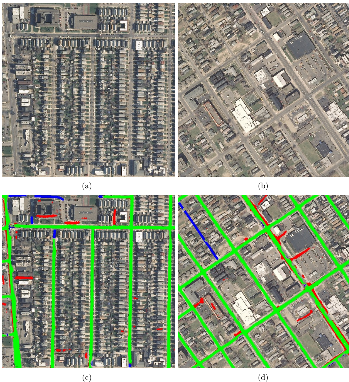
Figure 6.3: Figures 6.3(a) and 6.3(b) show two representative regions from the Massachusetts Buildings dataset. Figures 6.3(c) and 6.3(d) show predictions of a post-processing network on these regions.
