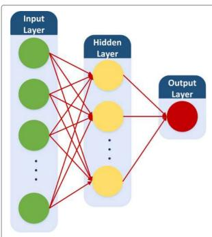
**Fig. 3** Conceptual structure of feed forward neural network with three layers
