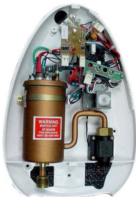
Figure 4.3: A Typical Water Heater Configuration
