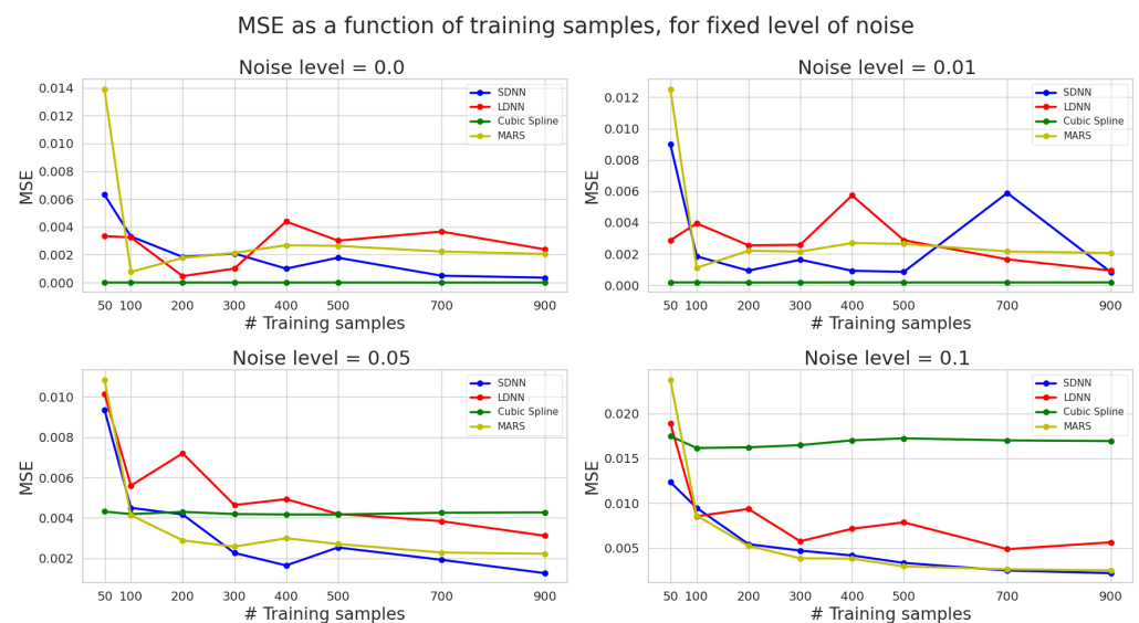
Figure 6. Test mean squared error vs. the total number of training samples for four different noise levels. The average values over five runs are presented. Blue represents SDNN, red LDNN, green cubic splines, and yellow MARS.
