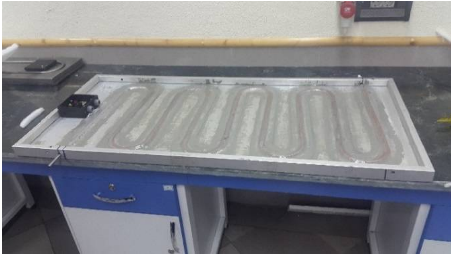
Figure 5. The PVT plate after connecting half-pipe
