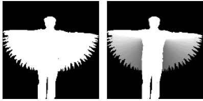
Fig. 7. Temporal templates similar to [30]. Left: motion energy image of a sequence of a person raising both hands. Right: motion history image of the same action.
