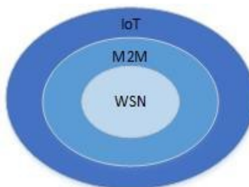
Figure 1 The relationship between WSN, M2M and IoT (see online version for colours)
