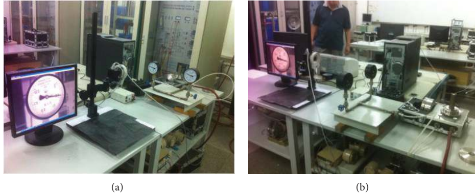
FIGURE 16: The experimental system of gauge test.
