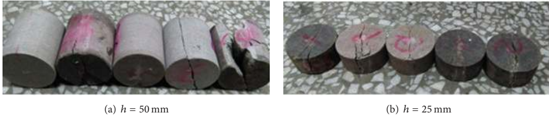
FIGURE 10: The damage form of sandstone after splitting test.
