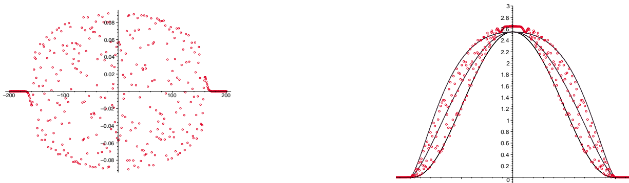
Figure 6.2: The dipole solution at t = 200 : displacement (left) and energy distribution (right).
