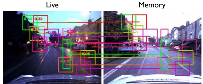
Fig. 1: We present an alternative to traditional point-feature localisation systems. Our system extracts distinctive elements from the environment using an unsupervised mining technique. We present a comprehensive N-vs-N analysis on 205 km of driving in central Oxford, showing that the proposed system is significantly more robust to appearance change than traditional approaches.
