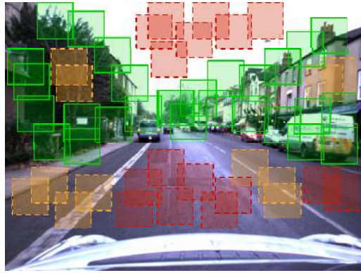
Fig. 3: Our unsupervised mining algorithm iteratively prunes and retrains a bank of robust detectors. The first phase trains a set of seed detectors (green, red and orange). By triangulating the landmark observations across a set of nearby images, we can reject landmarks which do not optimise to a consistent position (shown in red). A test for aliasing over a larger radius from the origin removes detectors which are not unique within the environment (shown in orange). The remaining detectors (shown in green) are saved.
