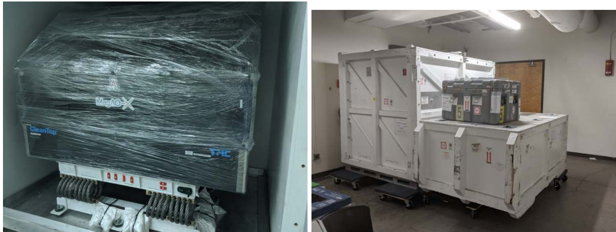
Figure 3. The MagAO-X shipping system. At left, the MagAO-X table assembly sits on the wire-rope isolator frame which safely transports the opto-mechanical system. At right: the entire MagAO-X system, including electronics and operator computer, in the shipping boxes awaiting transport.
