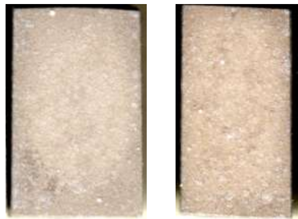
Fig. 7. Surface appearance of the anodised AZ31 samples after 15 days immersion in Hank's solution.
