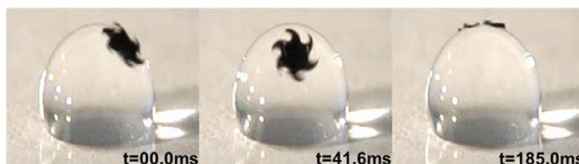
Fig. 11 A magnetic gyromixer in magnetic digital microfluidics. Reproduced from Ref. 93 with permission from Springer.
